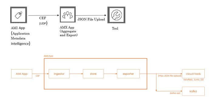
The AMX application can be deployed only on a GigaVUE V Series Node and can be connected to Application Metadata Intelligence running on a physical node or a virtual machine. The AMX application and the AMI are managed by GigaVUE-FM.
